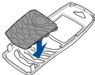
4. To attach the front cover, first place the phone and the front cover properly together and then gently push on the bottom and the top of the phone until the catches are locked properly.
