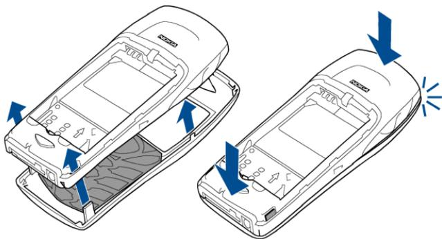
5. Slide the back cover into its place. See step 6 in Installing the SIM card and the battery on page 24.
