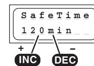
When you initiate a charge process, the integral safety timer automatically starts running at the same time. Its purpose is to prevent massive overcharging of the battery if the pack is faulty, or if the cut-off circuit is not triggered correctly.
